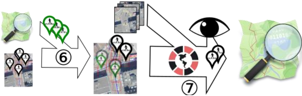
Figure 11: Detected crosswalks close to each other are merged, and those close to existing ones in OSM are eliminated (6). The remaining crosswalks are vetted by MapRoulette volunteers and manually added to OSM if deemed genuine (7).
