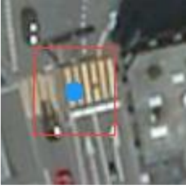
Figure 5: Visualization of the training data selection. The position of a crosswalk in OpenStreetMap is indicated by a blue dot. The red square is the border for the 50×50-pixel section to be cropped out of the aerial imagery
